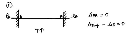
Here compatibility may be termed as continuity or good fit of material or structure or member or joint while being deformed under floading. Compatibility eg not satisfy because support connet be lifted. Now B joint is not continous.
